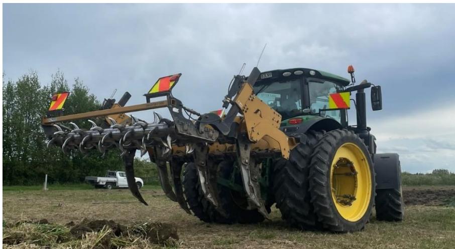
Figure 20 Ripper and incorporator used for conventional treatment.
