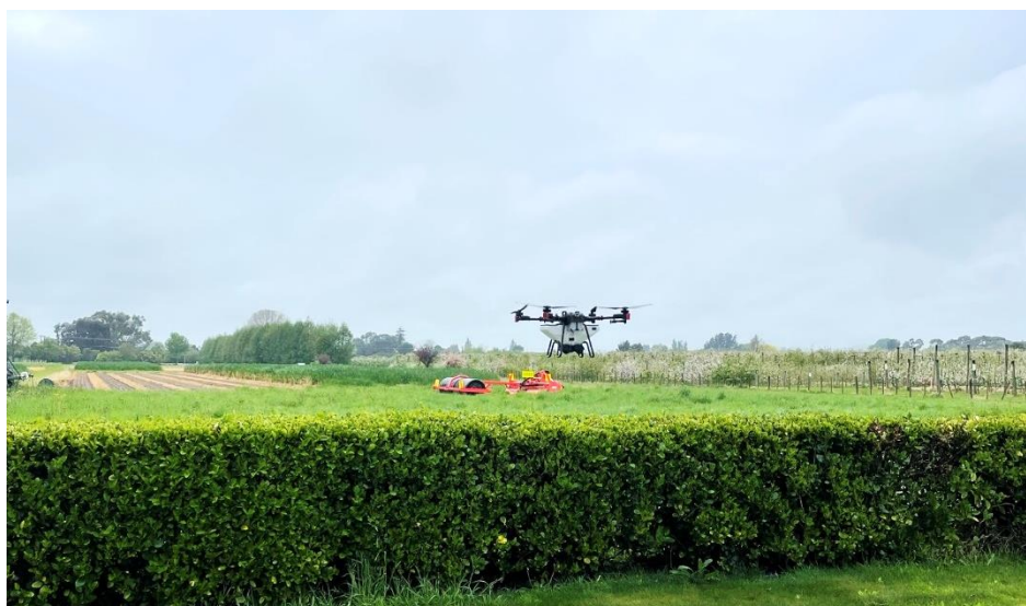
Figure 8 Airborne Solutions large drone used to apply lime, humates and micronutrients
