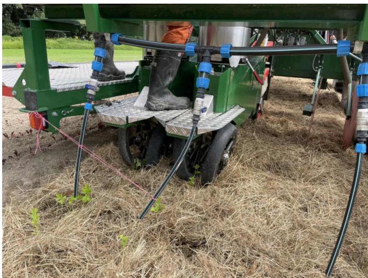
Figure 20 The Mulch-Tech planter being considered for establishing tomato seedlings in the regenerative treatment
