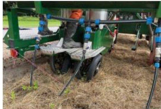
The MulchTec planter from live2give was tested and found suitable for planting tomato seedlings through thick residue mulch
